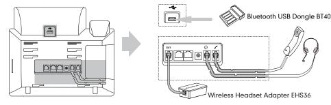
Note: The headset, Bluetooth USB dongle BT40 and wireless headset adapter EHS36 should be purchased separately. The EXT port can also be used to connect the expansion module EXP40. For more information on how to use the EHS36, EXP40 and Bluetooth USB Dongle, refer to Yealink EHS36 User Guide, Yealink EXP40 User Guide and Yealink Bluetooth USB Dongle BT40 User Guide.
