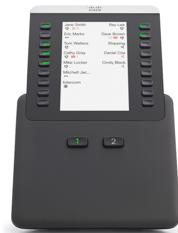
Figure 29: Key Expansion Module with Two Columns
